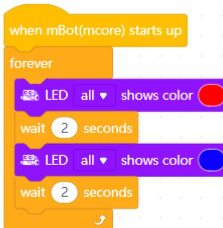
**Task 1:** Set the mBot LEDs so that each of the diodes (both left and right) lights up in a different color and changes to a different color after two seconds.
